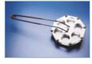
action handle is 38cm (15") long with a soft vinyl-coated grip. The handle also doubles as tongs for picking up hot crucibles. The octagonal carrier measures 203mm (8") across corners x 25mm (1") high with 48mm (1 15/16") diameter wells. Carrier includes handle/tongs. STAINLESS
